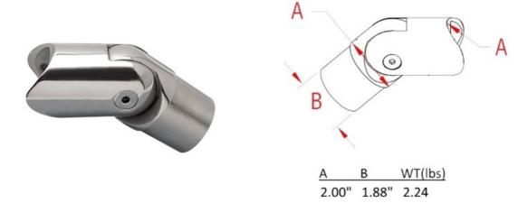
This adjustable elbow is made of 316 grade stainless steel, has a satin (brushed) finish, and is designed to mount on the **outside** of a 2" OD tube on one side of the fitting. The other side of the fitting is designed to fit **inside** a 2" OD tube with a 0.06" thick wall. Mount the first side with a fastener or by welding. Connect the second side with adhesive.
